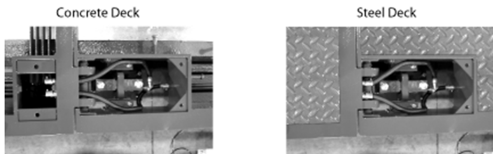
Figure 5-5. Conduit Connection Between Deck Modules
